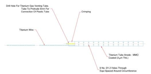
ISOMMO Discrete Anodes are supplied in the above standard dimensions. Each anode is supplied with a 700 mm long titanium wire feeder.
