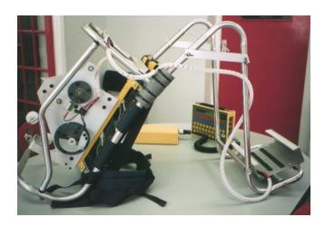
The carry frame comprising of the Surveyor Bac-Pac, Distance Measurement and Cable Dispenser System, has been specially designed to integrate with the Surveyor Data Logger to provide a comprehensive Data Input and Instrument Interface, thus enabling one man operation.
