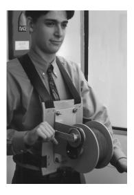
To facilitate efficient recovery and recycling of the BAC Surveyor wire the unique BAC Rewind System is available. Sturdily built, the rewinder allows the wire to be collected rapidly in the field and so be reused immediately.
