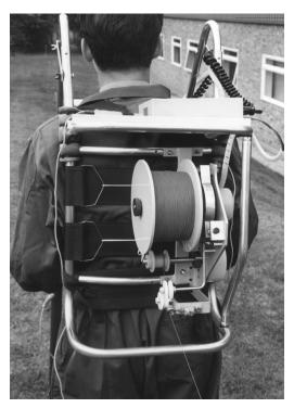
The reels and wire are robust and re-usable and when used with the **BAC Rewind System** provide a simple and cost effective cable recovery system.
